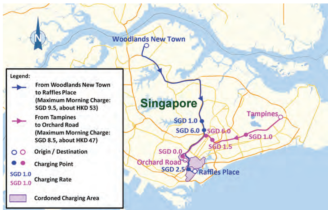
Figure 4.4 – Charges under two different routes in the Singapore Scheme
