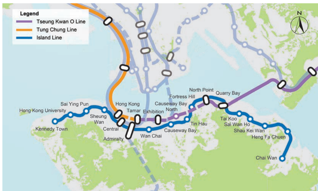
Fig. 4.7: Preliminary Conceptual Scheme of the “Interchange” Scheme of the North Island Line (Assuming Tamar as the interchange station)
